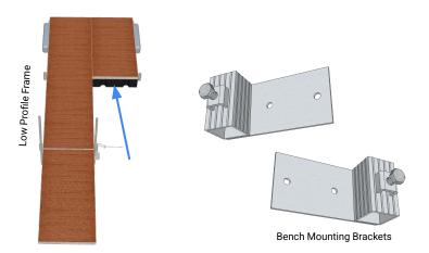
Mounting the Bench depends on the type of frame you have. The Low Profile Frame requires the Bench Mounting Kit (N8). The Bench Mounting Kit can be discarded for truss applications as the Bench directly mounts to the frame.
