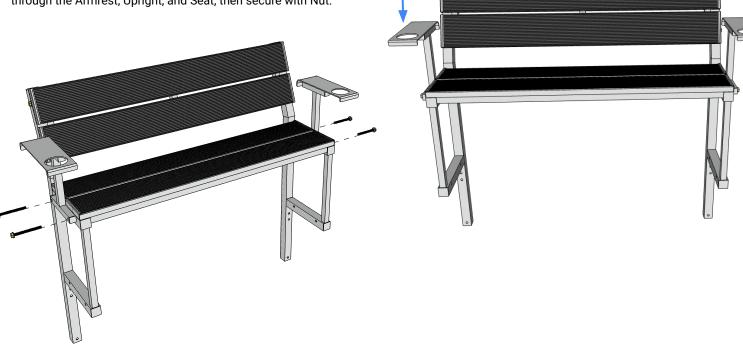
Firmly tighten all bolts including, Seat, Backrest, Mounting bolt for Truss, and Pinch Bolt for Low-pro.
