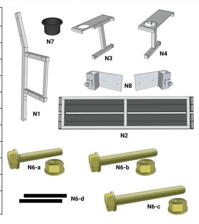
Apply both Rubber Strips (N6-d) to Bench Frames (N1). The strip will adhere to the BOTTOM of the square where it will rest on the decking.
