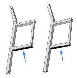
Select the location for the Bench on your frame. For both Truss frames and Low Profile frames, the bench typically mounts to the 4ft side of the dock frame, facing out toward the lake. Holes are pre-drilled in both frames for this location. There are also pre-drilled holes in the Low Profile frame along the 8ft side. Alternate locations can be drilled.
