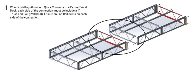
Install Female (B) Quick Connects to the supported side of the joint. Male (hook) Quick Connects will be installed on the non-supported side of the joint. Quick connects will share assembly hardware with PN10800 Patriot Dock Frame.
