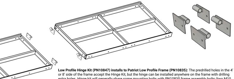
extra holes. Hinge kit will generally share some mounting bolts with PN10835 frame assembly bolts (two M10 bolt/nuts). Note: the round receivers are oriented upward.
