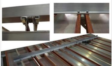
When installing Aluminum Deck Panels, first apply the adhesive backed Rubber or Cork Insulator to the aluminum frames. The Insulator is installed down the length of the 8' Side Rails and down the length of the Center Support Tubes. (Only used with Aluminum Decking) The Rubber/Cork Insulator is not to be installed in the direction of the 4ft. width, only lengthwise.
