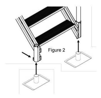
2 Insert Drop Leg and Base (C) into the bottom of each Stair Stringer (A). Secure with pinch bolt as shown in Figure 2. Drop Legs have roughly 5" of adjustment. Remember this will increase the rise of your first step. Adjust to desired height.
