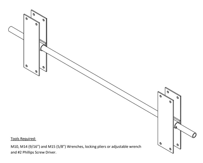
\*NOTE\* Each Patriot frame being joined together by the hinge must have a PN10803 End Rail installed on each side of the joint.
