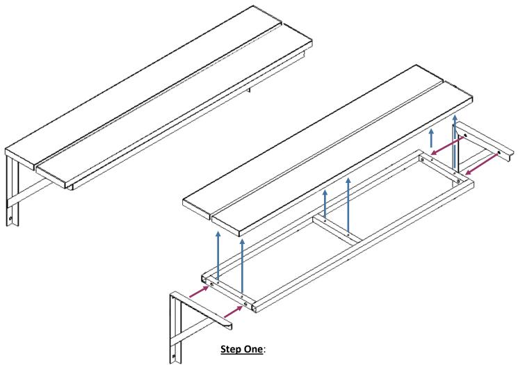
Left and Right Support Brackets are bolted to the rectangular aluminum frame using four M10x40mm bolts/nuts (red arrows)
