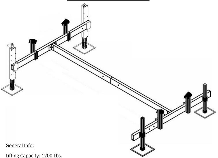
Frame Length: 96" Frame width: 60" or 72" Beam: 50" (64" with extensions)
