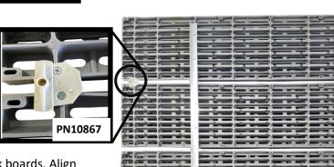
To assemble the **poly deck panel**, lay out deck boards. Align stringer with pre drilled hole on bottom side of poly board. Roughly 11-3/4" from edge. Secure with included screw.
