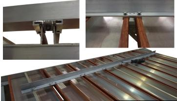
When installing Aluminum Deck Panels, first apply the adhesive backed Rubber or Cork Insulator to the aluminum frames. The Insulator is installed down the length of the 8' Side Rails and down the length of the Center Support Tubes. (Only used with Aluminum Decking) The Rubber Insulator is not to be installed in the direction of the 4 ft. width, only lengthwise.
