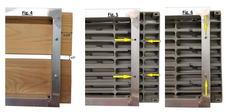
Step 3: After decking has been attached to the Aluminum Bench Supports using phillips head screws, the Aluminum Bench Supports can be set in place and attached to the Aluminum Uprights using the M10 x 100mm bolts, nuts and washers. See (Fig. 6).
