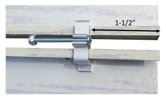
After the deck panel has been set in place on the Patriot dock frame, reach under and push the machine screw into place underneath the aluminum angle of the dock frame.
