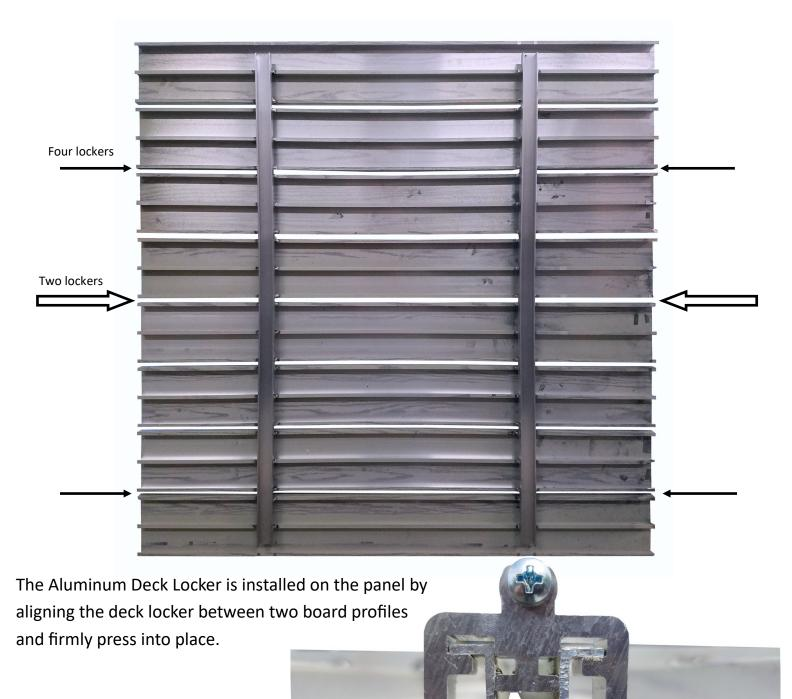
Slide Deck Locker at least 2" onto the aluminum deck panel, leaving approximately a 1-1/2" space from the edge of the panel to the outside edge of the Deck Locker.
